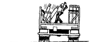
N.B. Some cylinders have a slightly more rounded base profile. These cylinders are relatively unstable compared to other cylinders. Extra care should be taken when handling them.
